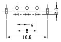
Recommended PCB Layout Top View
