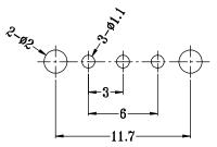
Recommended PCB Layout Top View
